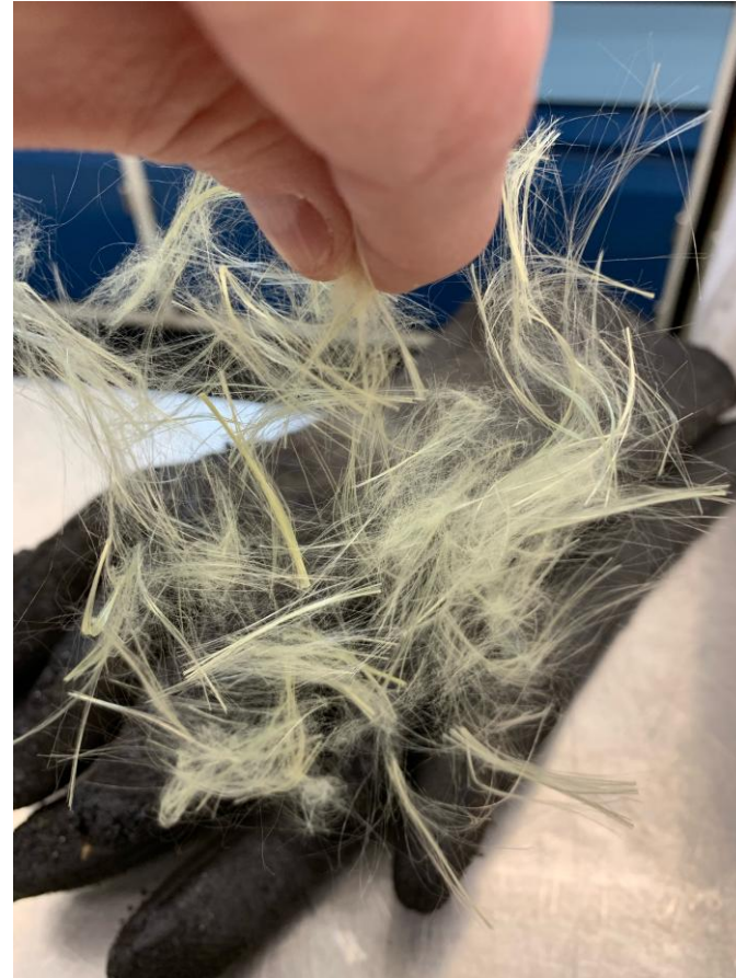
38mm aramid to ASTM D8395-23
